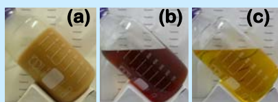
Photographs of (a) acid oil, (b) effluent from 1st column with PK208LH and (c) effluent from 2nd column with PA306S
