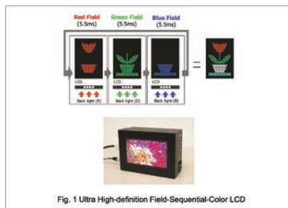
Fig. 1 Ultra High-definition Field-Sequential-Color LCD
