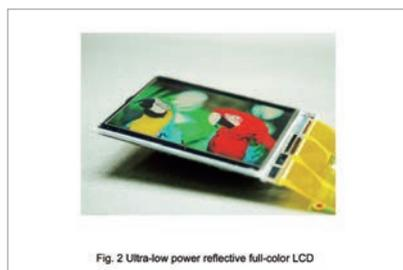
Fig. 2 Ultra-low power reflective full-color LCD
