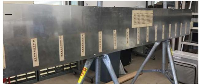
Antenna for 17GHz MIMO-Type GB-SAR
